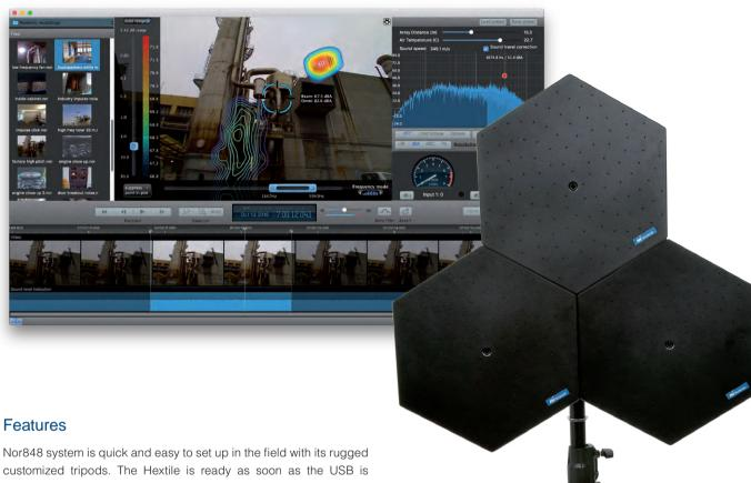
Nor848 system is quick and easy to set up in the field with its rugged customized tripods. The Hextile is ready as soon as the USB is plugged and the application is launched. The Multitile, with its three Hextiles and a bigger tripod, is set-up and ready to measure in less than five minutes.
